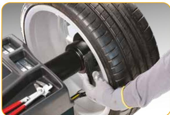
**EN** → **Size detection** Automatic acquisition of distance, **28"** diameter and wheel width with integrated **QP (Quick Program)** function that automatically activates the balancing programmes avoiding the use of the keyboard. Three systems for positioning adhesive counterweights: assisted with weight holder clips or manually at **6 o'clock** or at **12 o'clock**.
