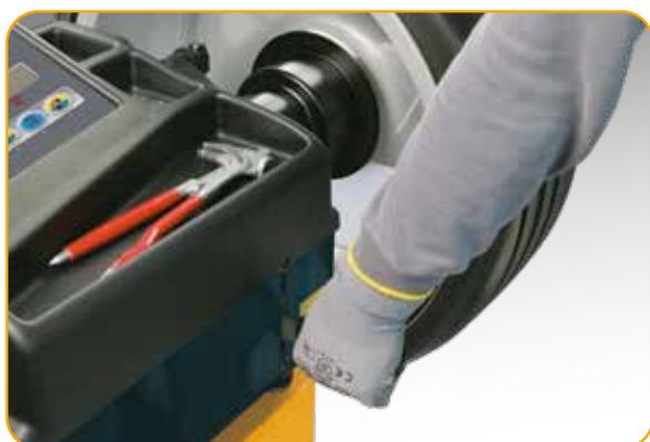
**EN** → **Clamping brake** It makes wheel clamping and unclamping operations and counterweight application easier. The lever, in motorised versions, also allows running the spin motor at 100 rpm.
